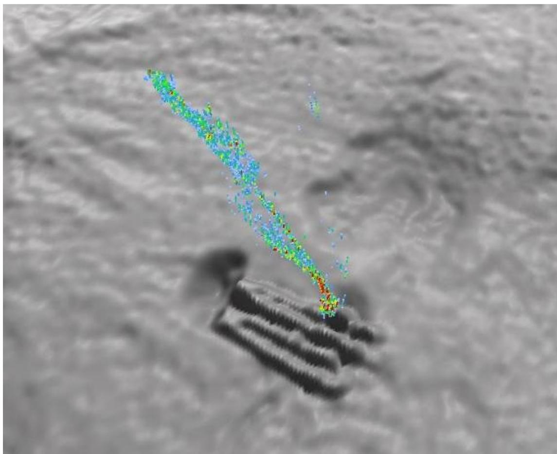
Exhibit 1A: Image from the NOAA R/V *Okeanos Explorer* vessel-of-opportunity multibeam sonar survey over the MC-20 site in June 2012, showing an oil and gas water-column anomaly over the northeastern side of the jacket.
