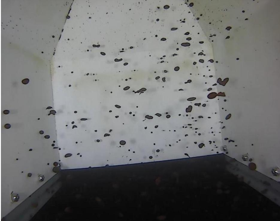
Exhibit 5: Screen shot from the NOAA/BSEE 2018 bubbleometer video showing the oil droplets being released from the oil-only plumes emanating from the pit near Dome C. For reference, the pan-head machine screws shown in this figure were 1/4" (6.35 mm), and have 7/16" (11.11 mm) lock nuts on the inside of the housing. A video clip is attached separately.
